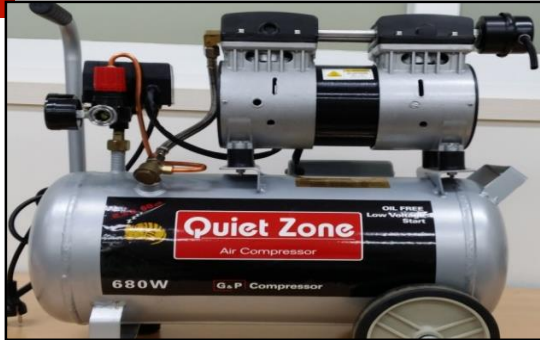
Air Compressor : 1.0[Hp]/10l Electricity 220V
