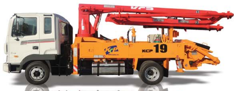
KCP19Z80 BOOM HEIGHT 18,1 m BOOM SECTIONS 3 MAX. OUTPUT 70 m 3 /h
