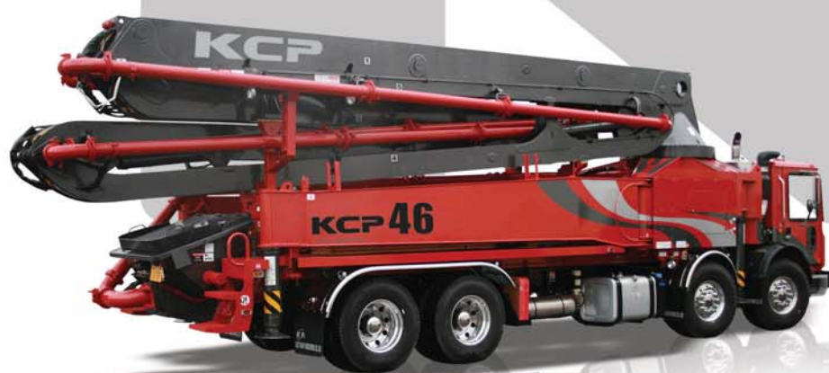
KCP46ZK170 BOOM HEIGHT 45,3 m BOOM SECTIONS 5 MAX. OUTPUT 170 m 3 /h
