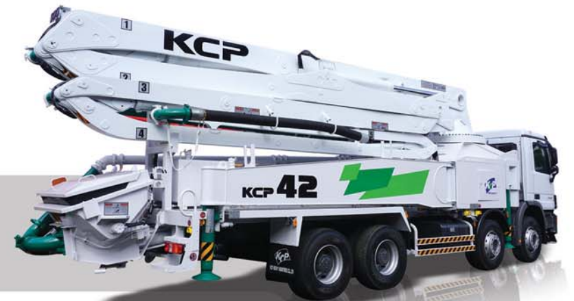
KCP42ZK5170 BOOM HEIGHT 41,4 m BOOM SECTIONS 5 MAX. OUTPUT 170 m 3 /h
