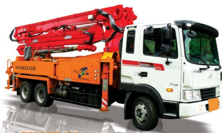
KCP28Z100 BOOM HEIGHT 27,1 m BOOM SECTIONS 4 MAX. OUTPUT 100 m 3 /h
