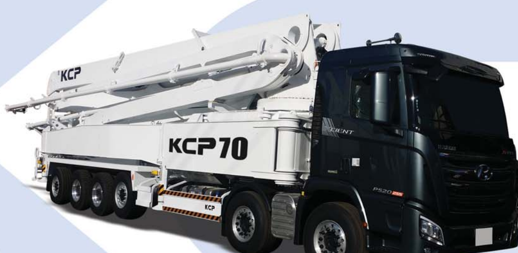
KCP70ZS170 BOOM HEIGHT 69,45 m BOOM SECTIONS 5 MAX. OUTPUT 170 m 3 /h
