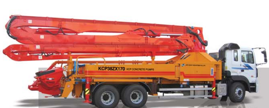
KCP38ZK170 BOOM HEIGHT 37,8 m BOOM SECTIONS 4 MAX. OUTPUT 170 m 3 /h
