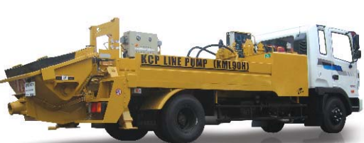
KML 90H MAX. THEO. HORIZONTAL TRANSFER 315 m MAX. THEO. VERTICAL TRANSFER 180 m CONCRETE PRESSURE 147(H)/99(L) bar MAX. OUTPUT 80
