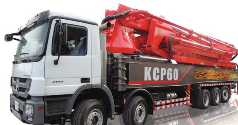
KCP60ZS6170 BOOM HEIGHT 59,6 m BOOM SECTIONS 6 MAX. OUTPUT 170 m 3 /h
