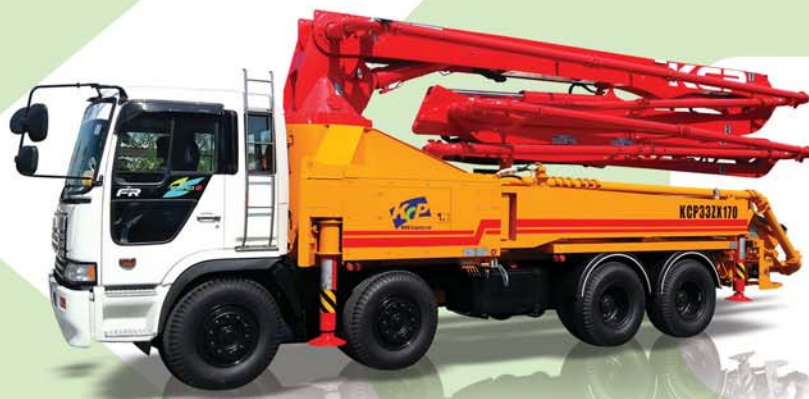
KCP33ZK170 BOOM HEIGHT 32,1 m BOOM SECTIONS 4 MAX. OUTPUT 170 m 3 /h
