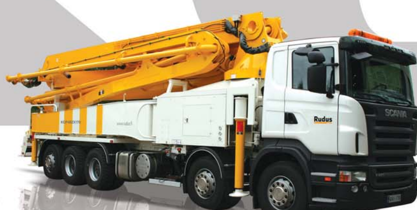
KCP48ZK170 BOOM HEIGHT 47,1 m BOOM SECTIONS 5 MAX. OUTPUT 170 m 3 /h
