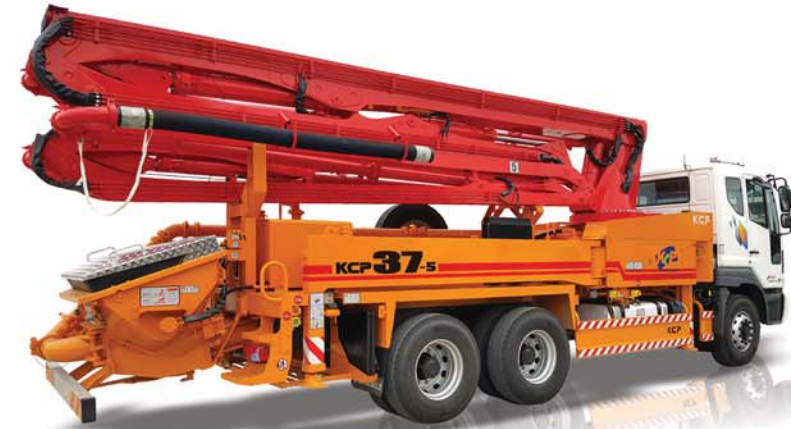
KCP37ZK5170 BOOM HEIGHT 36,34 m BOOM SECTIONS 5 MAX. OUTPUT 170 m 3 /h
