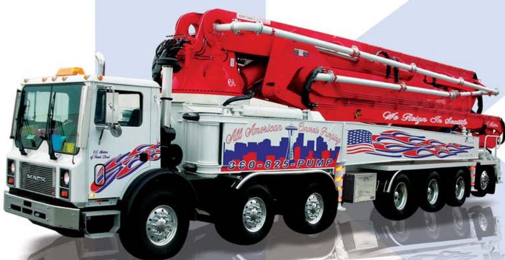
KCP65ZS170 BOOM HEIGHT 64,4 m BOOM SECTIONS 5 MAX. OUTPUT 170 m 3 /h
