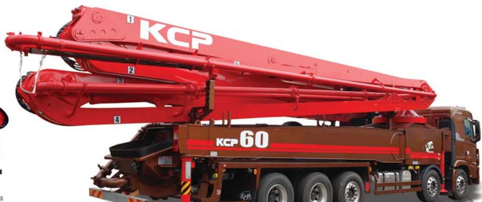
KCP60ZK170 BOOM HEIGHT 58,5 m BOOM SECTIONS 5 MAX. OUTPUT 170 m 3 /h
