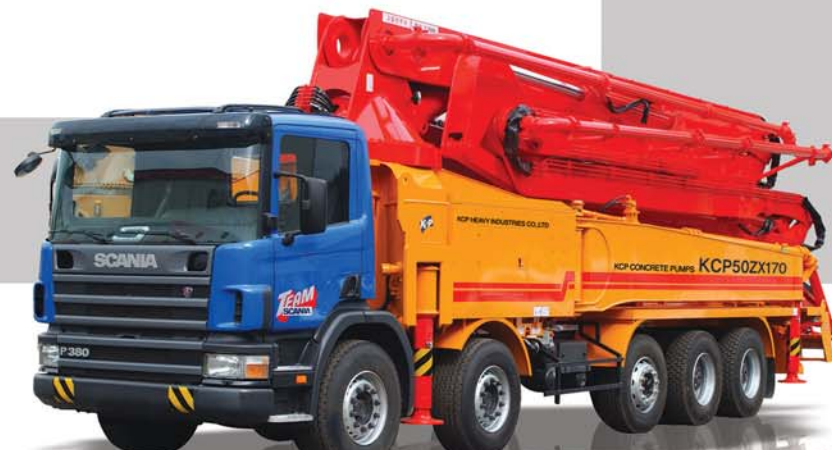
KCP50ZK170 BOOM HEIGHT 49,4 m BOOM SECTIONS 5 MAX. OUTPUT 170 m 3 /h
