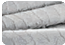
When using regular detergent (some damage, such as rip)
