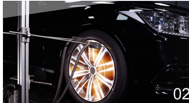
Chassis Noise Dynamometer
