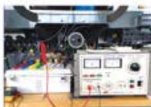
High Potential Voltage Test
